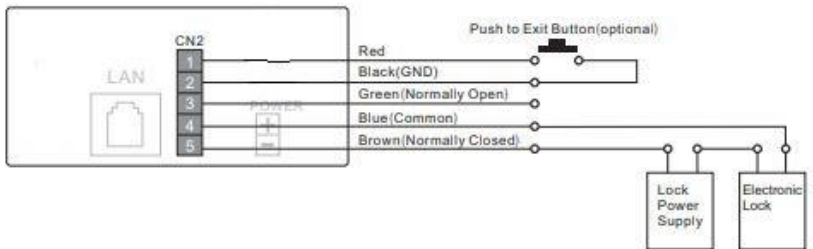
Wiring Diagram for Normally Closed Circuit (e.g. Electronic Mag Lock)
